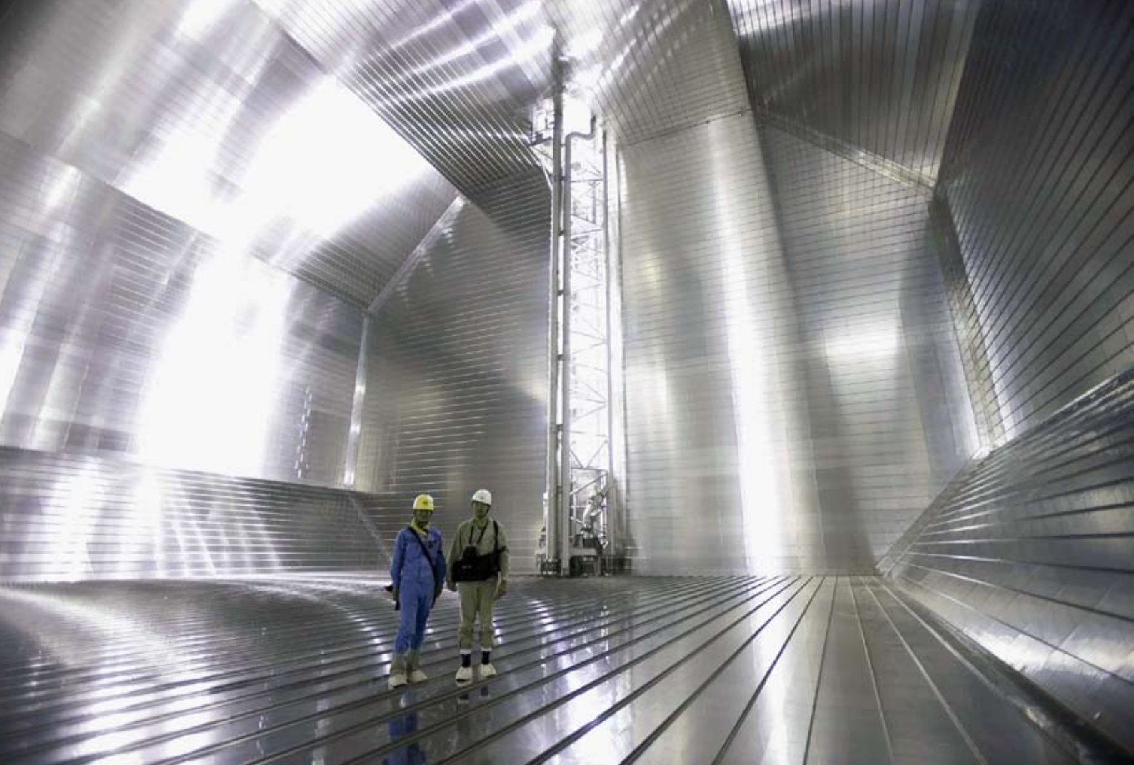
Inside an LNG tanker which is made of Fe-36%Ni alloy.
