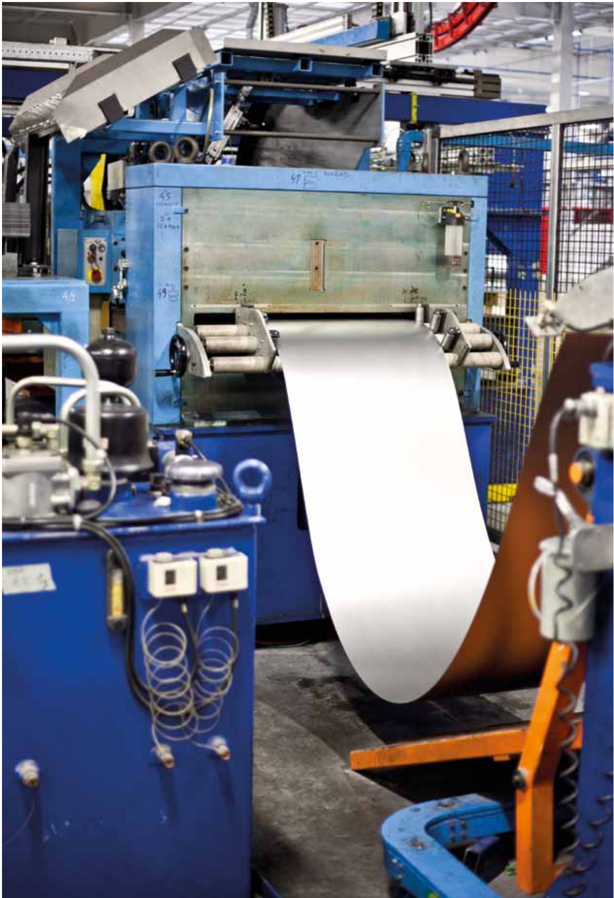
The first station of the housing manufacturing line – sheet metal straightening device
