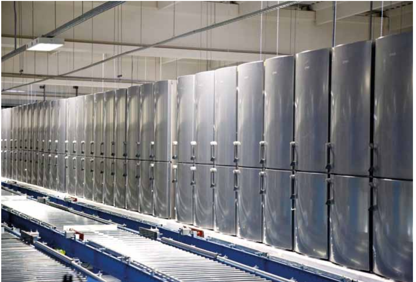
Transport of final products to the 100% clean chamber for safety characteristics and operation testing
