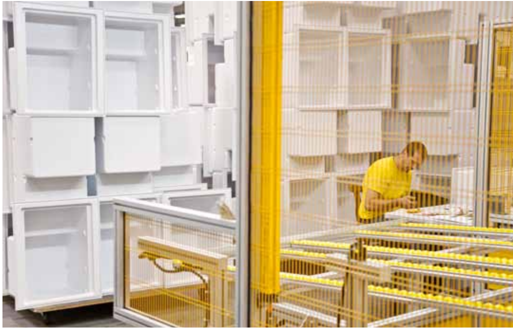
Outgoing conveyor of inner liner cut-out device
