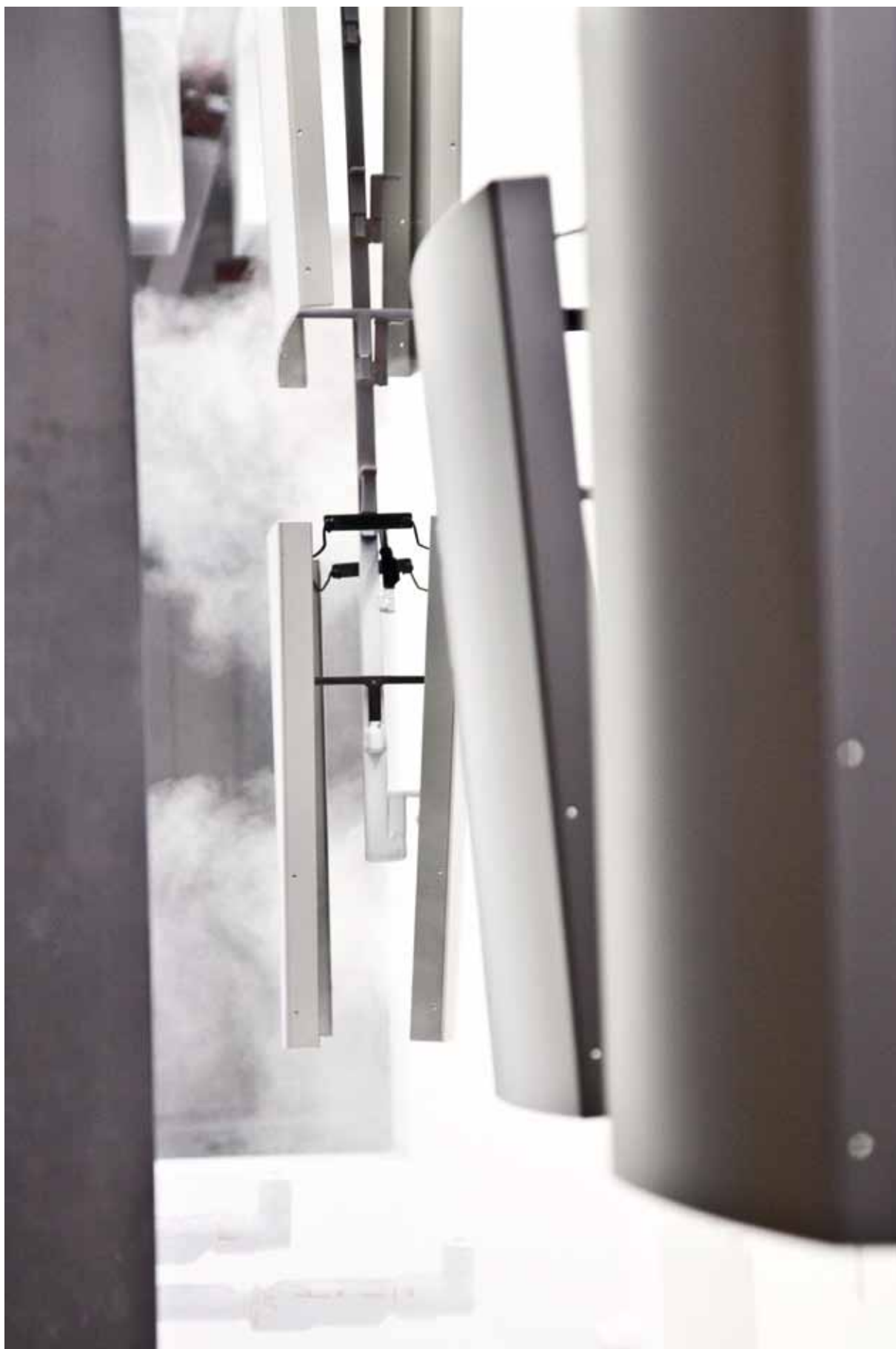
Powder coating process in special powder coating chamber
