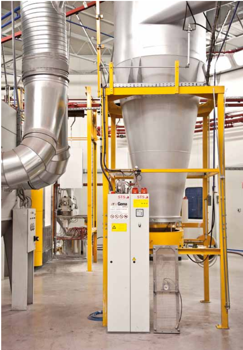
A cyclone; separation of the dust that remains in the process of powder coating
