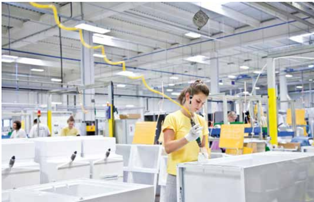
Preparation of inner liner (refrigerator interior) for installation into the housing in the pre-assembly section
