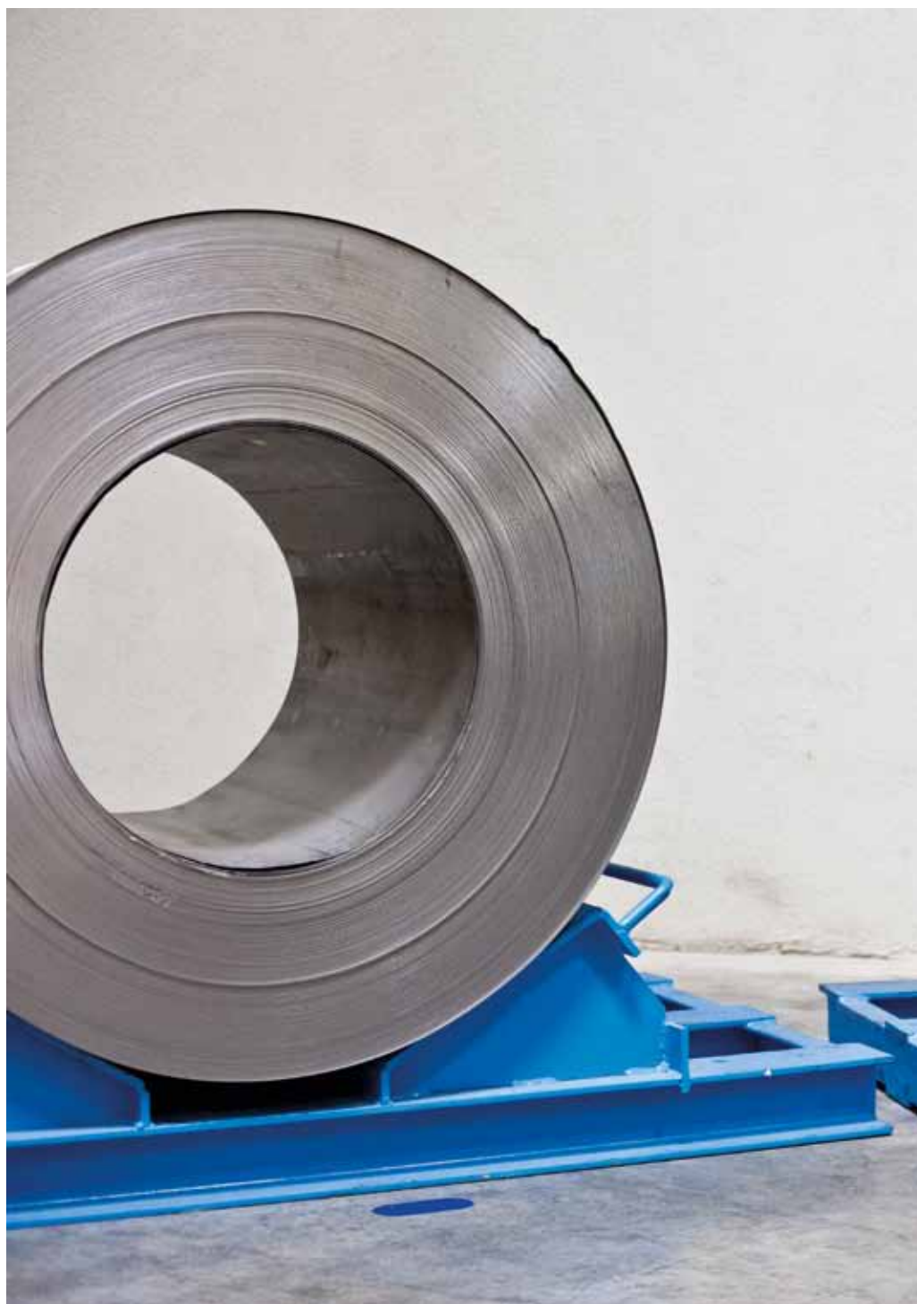
Rolls of sheet metal for doors and cabinets
