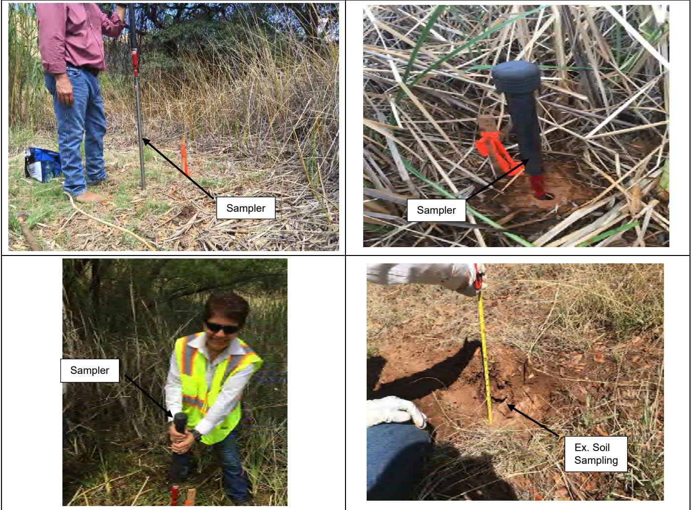
Photo 3: Sampling using AMS Replaceable Tip San/Loose Sediment Probe and Existing Soil Grab Sample
