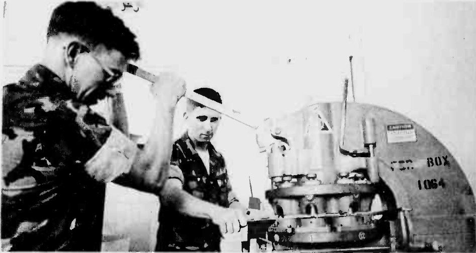
POWER PUNCH — Sergeants Rodney Collins (left) and Maintenance Squadron-24's Metal Shop. (Photo and Phil Martin team-up to make a few holes in a piece of metal with a turret machine at Headquarters) (Photo by Sgt Chris Taylor)
