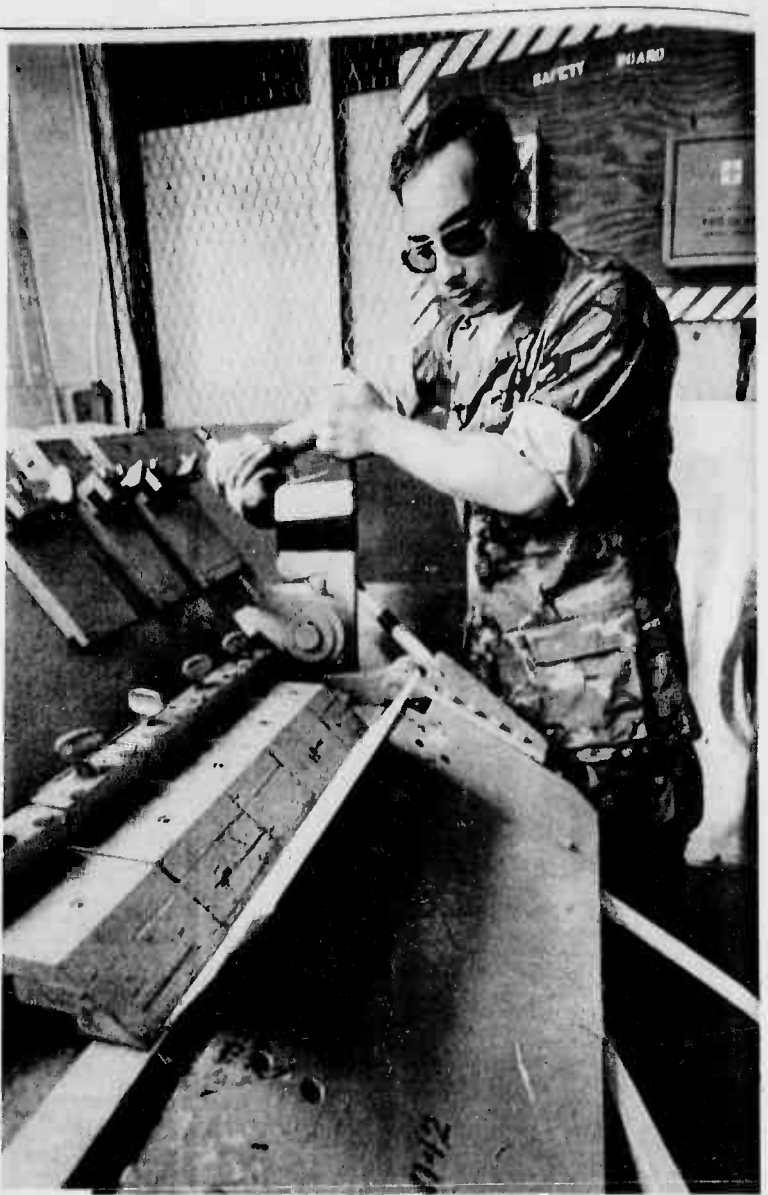
CORRECT ANGLE — Corporal Frank Burgos forms an angle with the help of a brake machine. The metal-shaping machine is one of the machines used at Headquarters and Maintenance Squadron-24's Metal Shop. (Photo by Sgt Chris Taylor)
