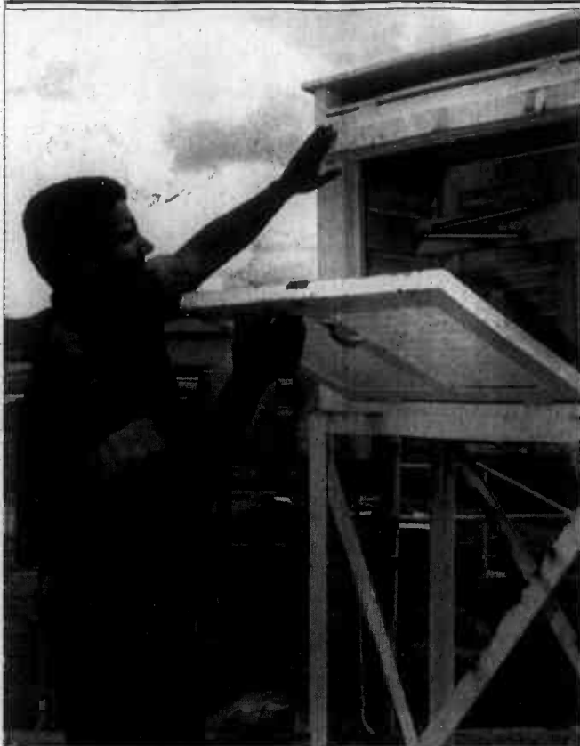
Lt. Jose Hernandez, weather observation specialist, Weather Service Office, Marine Corps Air Facility here, opens a thermoscreen to check weather instrumentation housed inside.
