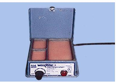
9.21.2. **Maintenance.** Clean the unit period ically to prevent accumulation of debris in the bottom of the wax compartments.
