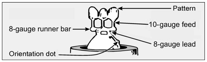
1.52.4.3.3. This spruing technique allows molten metal to be cast into the mold so it fills the mold uniform ly and simultaneously, thus elim inating variations that occur when m olten metal hits different areas of the mold at different times. Indirect spruing increases turbulence (over the direct m ethod) and reduces backpressure when the m etal is cast into the mold. It helps eliminate shrink spot porosity because the feed of molten metal stays open longer.
