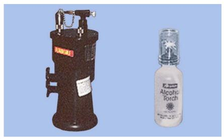
9.48.2. **Maintenance.** Check the nozzle tip to ensure it is free of obstructions. Replace the bellows diaphragm as needed. Clean the exterior of the pump daily to prevent accumulation of waxes and compounds.
