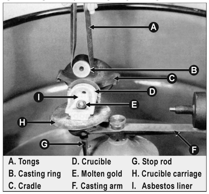
Figure 1.62. Melting the Gold Alloy and Positioning the Ring in the Casting Machine.
