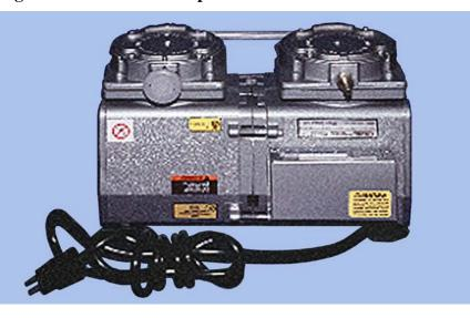
9.40.2. **Maintenance.** Read the manufacturer's recommendations for maintenance on each type of pump. Most pumps require the intake and exhaust filters to be periodically checked and cleaned. If applicable, the oil in the vacuum pump should be replaced every 90 days or any time a change in color is noted in the inspection eye.
