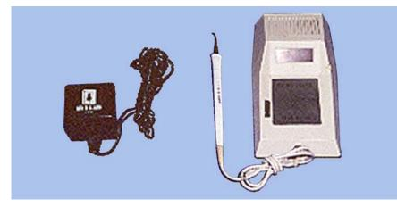
9.53.2. **Maintenance.** Never cover the top vent holes. Do not allow wax or debris to enter the unit through the vent holes. Only a qualified technician should open the unit for any repairs. Do not set the temperature higher than necessary. Do not use the stand ard waxing tip hold er above 450 °F. Keep the spatula tips clean and free of carbonized wax.
