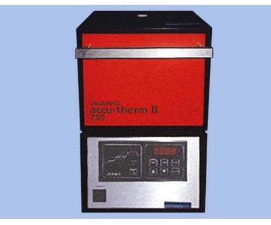
9.32.2. **Maintenance.** Clean the muffle of the burnout oven to rem ove all debris. Vacuum inside the muffle as required. Check the pyrometer of the oven every 3 months. Use temperature pills or a pure m etal to check for proper calibration. Never operate the burnout oven at higher temperatures than those recommended by the manufacturer. Keep the muffle door closed when the furnace is cooling because an open door leads to too rapid cooling which may crack the muffle.
