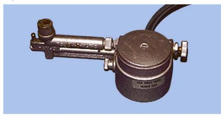
9.6.2. **Maintenance.** The burner has few m oving parts and requires little m aintenance. When wax or similar materials drop into the burner, rem ove the burner assembly from the unit and clean it in boiling water. After boiling and before reattaching the burner assembly, blow out any excess water from pilot tube, gas inlet tube, and flam e orifice. Be sure the sm all round O-ring attached to the projecting brass tubing of the burner is replaced before reassembly.
