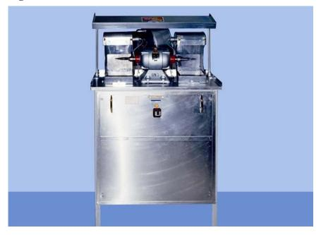
9.26.2. **Maintenance.** Dust and clean the m otor housing and unit daily. Replace the filters as required.
