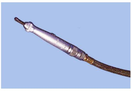
9.11.2. **Maintenance.** Do not atte mpt to operate the chuc k unless it is properly installed on the lathe. Never use oil or solvents of any kind on it. Never close the collet without a tool (chuck or bur) in the collet. Allow the clut ch spring to slowly engage the clutch. (Never push up on the handle or let the handle snap up.) Do not re move or attempt to defeat the purpose of the safety strap. Clean the collets once a week.
