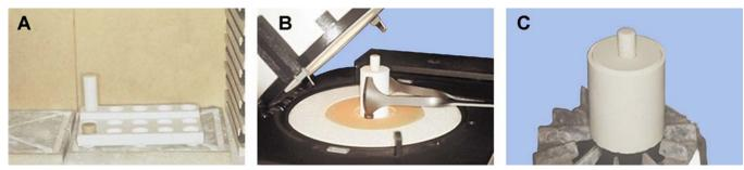
4.7.5.2. Remove the mold from the furnace with ope ning up and immediately place the ingo ts from the support tray into the hot mold. Place the alox plunger on top of the ingot, ensuring it is fully seated in the mold (Figure 4.10-B). Select the desired program . (Consult the manufacturer's pressing table for exact data.)
