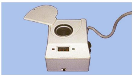
9.20.2. **Maintenance.** Never pry unm elted wax from the well because seve red amage to the silicone d iode tem perature senso r m ay result. Keep the wax well covere d when not in use. Periodically remove the cover and clean any excess wax that may have collected.
