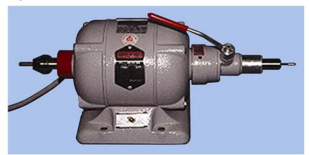
9.25.2. **Maintenance.** The bearings are factory sealed and require no lubrication. Do not flip the switch from "HIGH" to "LOW" to slow the m achine down. The chuck m ust be periodically cleaned and lubricated to prevent rusting and ensure its smooth function.
