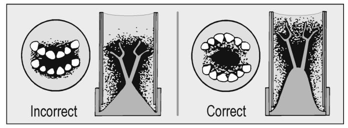
2.7.5. **Orientation Dot.** Besides depending on the force gene rated by a spring-wound casting arm to fill a burned-out mold, it is critical that the mold gets maximum benefit from the natural flow of
