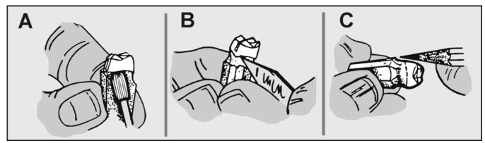
1.33.1.2.2. **Define the Margin.** Do the final trimm ing with a #25 Bard Parker blade or beaver blade. At the mesial and distal surfaces, make the cuts *straight down* because the proximal contours of patterns are fairly straight. On the facial and lingu al areas, s trive for about 0.5 mm of undercut. Defi ne only the gingival m argins, not those prepared as supragingival (above the gingival crevice, as in a 3/4-crown preparation).
