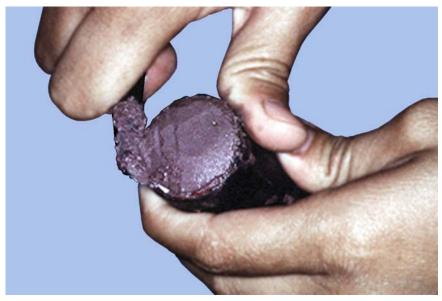
Figure 1.59. Breaking the Top Surface Glaze of the Set Investment.
