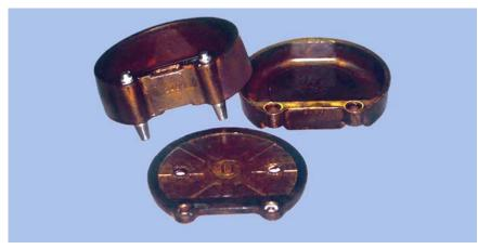
9.17.2. **Maintenance.** Clean and apply a lig ht coat of petrolatum to the flask after each u se. Always use the e jector press, not a metal hammer, to remove the molds. When the brass on the flask tarnishes, restore its appearance with fine steel wool or a fine emery cloth.
