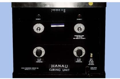
9.13.2. **Maintenance.** Check the electrical cord for wear or dam age. Ensure the unit has a grounding plug. Check the unit for water leaks in the tank or valve. Drain and clean the tank periodically, removing debris with a stiff brush (not a steel one) and cleaning solvent. Rem ove lime deposits by soakin g with ace tic acid (vine gar). Perform the following operational check at least monthly:
