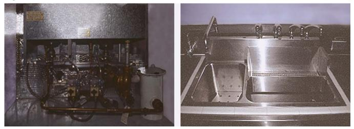
9.46.3. **Safety Considerations.** A lways wear safety glasses and heat resistant gloves when operating the tank. If, during the lig hting procedure, the pilot will not s tay lit after several tries, turn the gas completely off and call a service tec hnician. Stand clear of the facets when the pum p is turned on to avoid being burned by splashing hot water.
