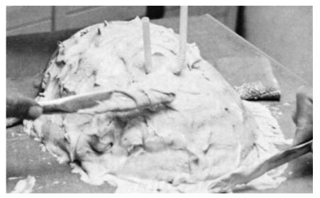
Figure 7.19. Supporting Stone Layer Completed to a Depth of 1/2 Inch.
