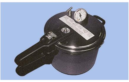
9.35.2. **Maintenance.** Periodically check seals, air in lets, and outlets for m alfunctions. Activate the pres sure relief valve to ensure it is operational. Periodically lubricate the g asket to prevent from drying out.
