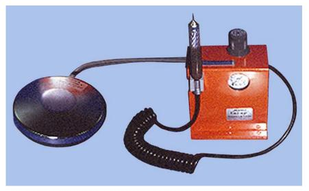
9.22.2. **Maintenance.** Never run handpiece without a bur in the chuck. Lubricate the headpiece after 3 to 5 hours of operation or at the end of each workday. (See the manufacturer's manual for guidance.) Always ensure burs are true before usi ng them. Ensure the air pr essure is set at the manufacturer's recommendation; higher air pressure could damage the handpiece.
