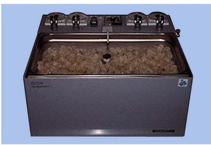
9.14.2. **Maintenance.** Periodically check the power cord for damage. At least monthly, perform an operational check to ensure water temperature is maintained at 100 °C. Always ensure there is an adequate number of insulation floaters to cover the water's surface. As se diment builds up, clean the tank with a brush and mild solvent.
