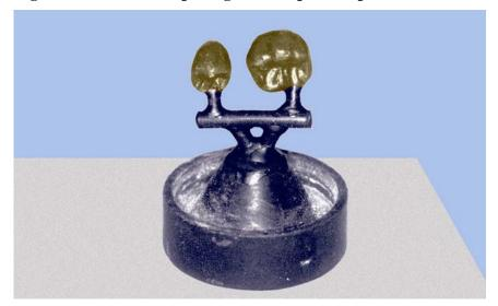
Figure 1.54. Indirect Spruing of Multiple Independent Patterns.
