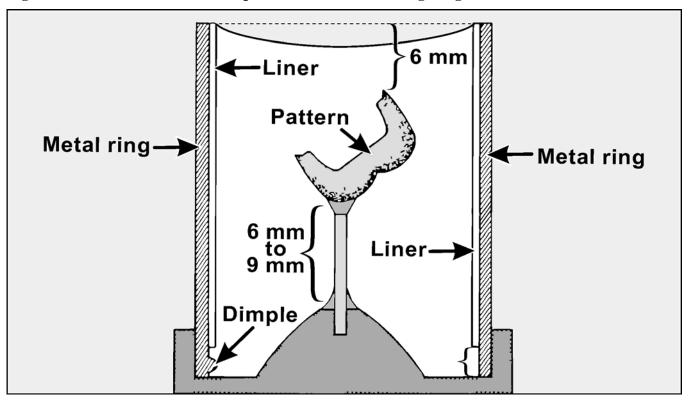
Figure 1.55. Schematic View of a Sprued Pattern in a Casting Ring.
