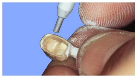
Figure 1.64. Pickling a Casting.
