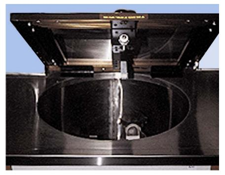
Figure 9.7. Broken-Arm Casting Machine With Safety Lid.
