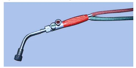
Figure 9.53. Gas and Air Casting Torch.
