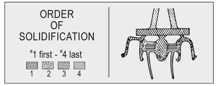
Figure 2.16. Placement of Chill Vents on a Substructure Pattern.
