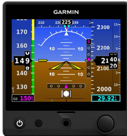
Figure 1-1 G5 Electronic Flight Instrument (Attitude)
