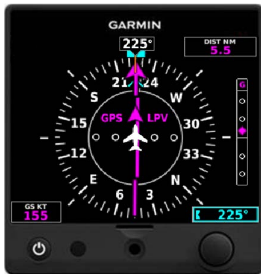
Figure 1-3 G5 Electronic Flight Instrument (DG/HSI)
