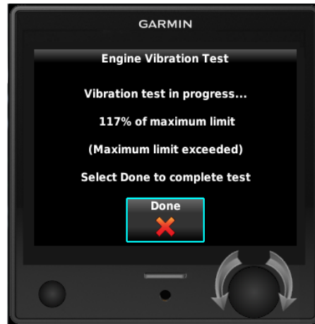
Figure 6-3 Engine Vibration Test Failure Indication
