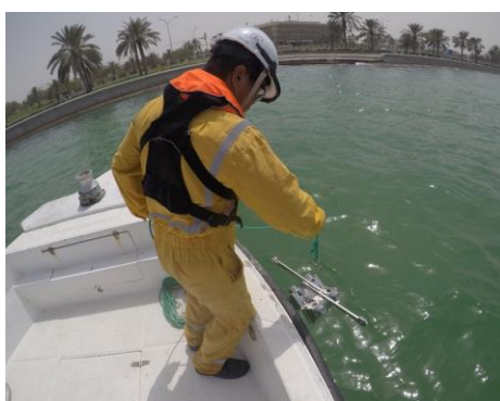
Figure 4 Marine sediment for chemical analysis and benthic infauna was recovered using a Van Veen grab
