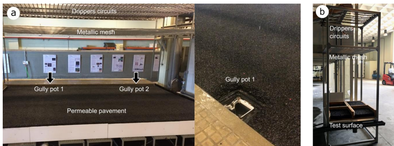
Figure 1. (a) Permeable pavement placed over a street section physical model of 36 m 2 and detail of the surroundings of gully pot 1. (b) Rainfall simulator of 1 m 2 for the analysis of the pollutant removal efficiency of the permeable pavement.
