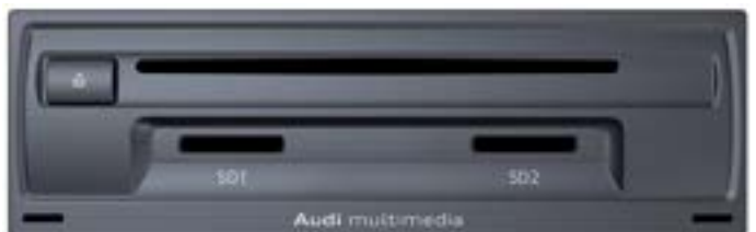
Front panel of J794 for High-spec MIB**
