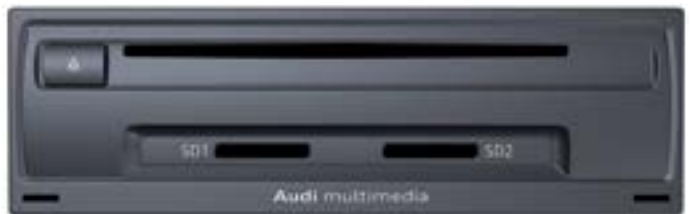
Front panel of J794 for Standard MIB, navigation system version
