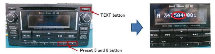
• If the 4th, 5th and 6th digits of the version ID number displayed are 504 as shown in the photo above, the unit must be updated. If they are 505 or higher and the system does not automatically display the **BT SEL LANGUAGE** screen, the audio unit will need to be replaced with an exchange unit from Clarion.
