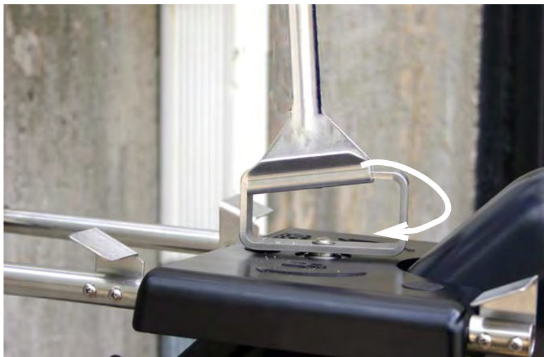
Figure 2-30 Turn the locking handle clockwise until sensor is locked into place (shown with the optional sensor retrieval arm, described in Section 2.8)
