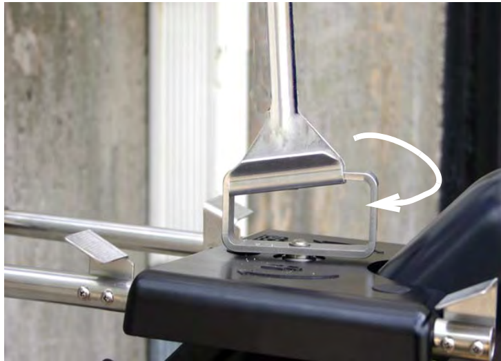
Figure 2-22 Turn the locking handle clockwise until sensor is locked into place (shown with optional sensor retrieval arm, described in Section 2.8)
