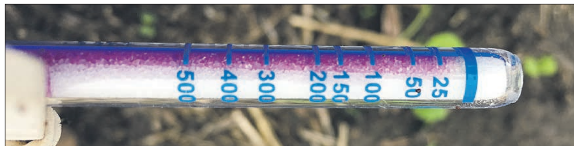
Dositubes, used to measure nitrogen volatilization losses, were placed under boxes with holes drilled in them on a recently seeded field shallow-banded with urea. The tubes contain purple packing material containing sulfuric acid that turns yellow when it reacts with the gas. | AGRITRUTH RESEARCH PHOTOS
