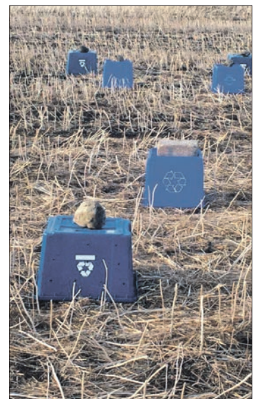
Dositubes, used to measure nitrogen volatilization losses, were placed under boxes with holes drilled in them on a recently seeded field shallow-banded with urea. The tubes contain purple packing material containing sulfuric acid that turns yellow when it reacts with the gas. | AGRITRUTH RESEARCH PHOTOS
