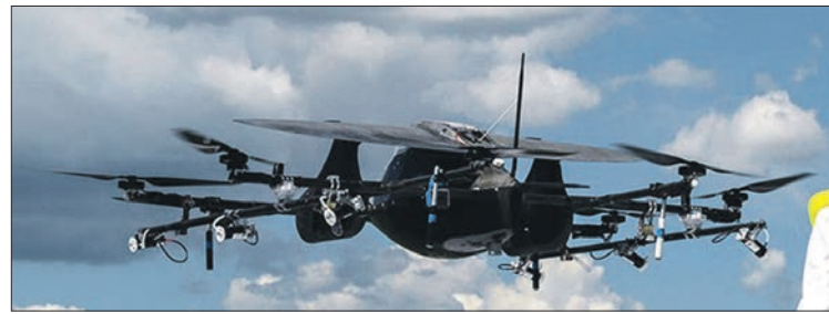
TOP: The Kray drone rotary atomizer nozzles are designed specifically for drones. | KRAY TECHNOLOGIES PHOTO
