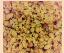
Microscope image of Anobium punctatum bore dust. Note that it is composed of lemon-shaped pellets that cause it to feel 'gritty' when rubbed between the fingers.
