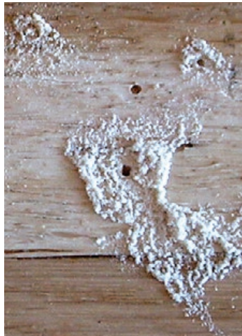
Note how the infestation is only affecting the sapwood of this oak section.
