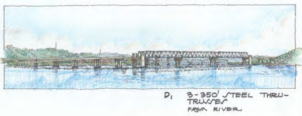
(e) D1–Three 350-Foot Steel Thru Trusses
