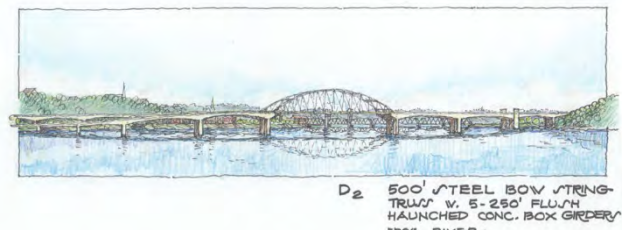
(f) D2–500-Foot Steel Bowstring Main Span with Five 250-Foot Haunched Concrete Girders
