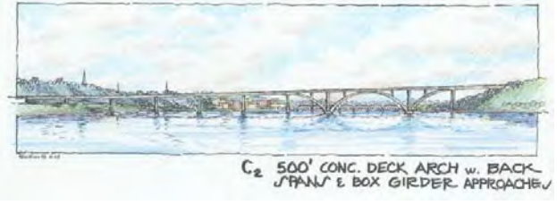
(d) C2–500-Foot Concrete Girder Arch and Box Girder Approaches
