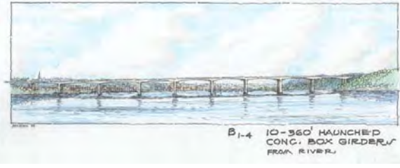
(c) B1-4–Ten 360-Foot Haunched Concrete Box Girders
