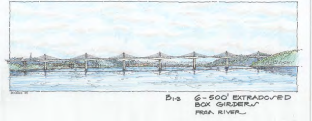
(b) B1-3–Six 500-Foot Extradosed Box Girders
