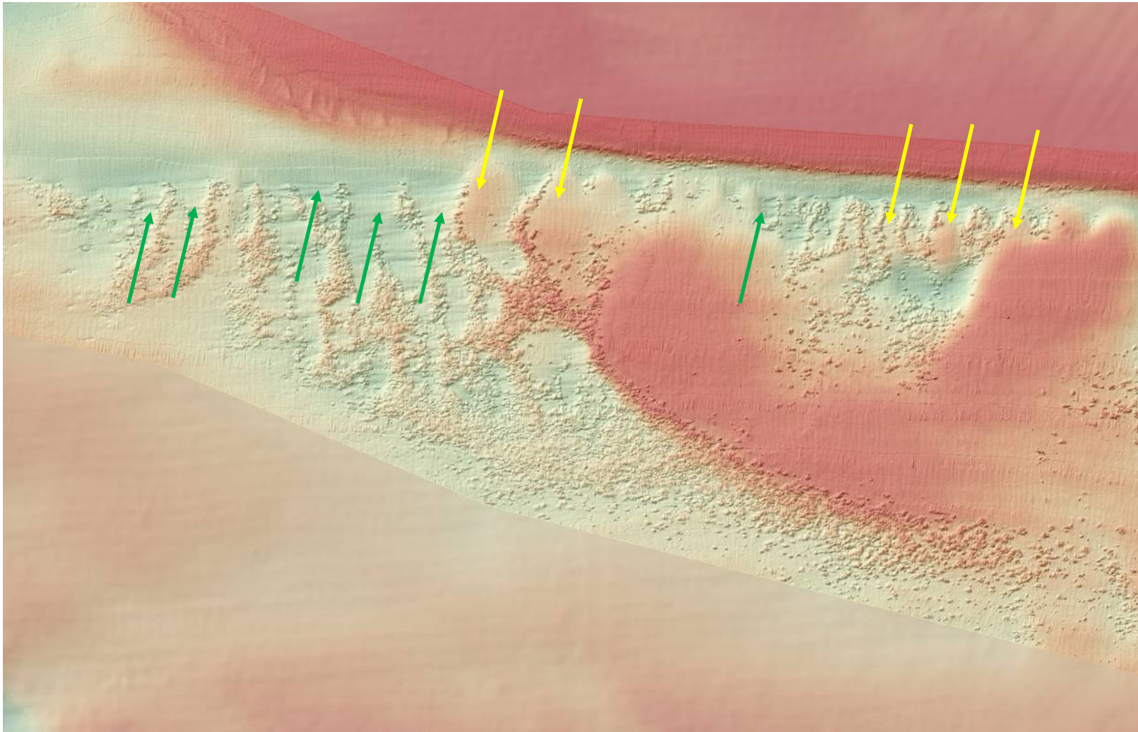
Figure 12 Potential sediment accretion on eastern sides of reef rows (yellow arrows) and scour (green arrows) on western sides. Colour gradient represents depth range 3.3 to 6.5 m.
