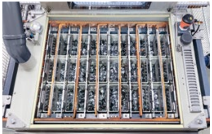
HelioChrome® NEO nugget dissolution cell
