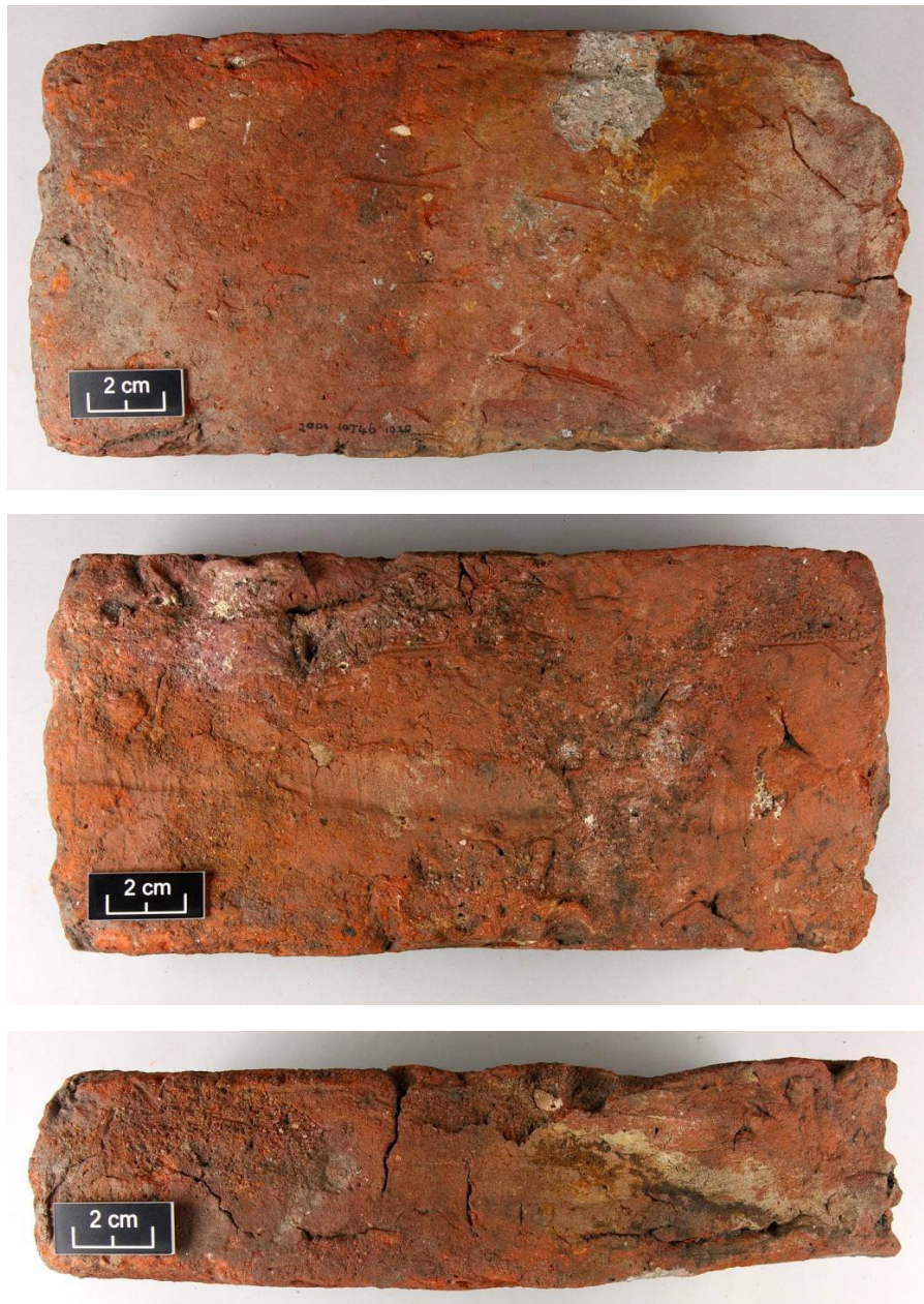
Plate 39: The upper bed, lower bed and one stretcher of a post-medieval brick from the excavations at St Leonard's Hospital, York A turning mark is visible on the central image
