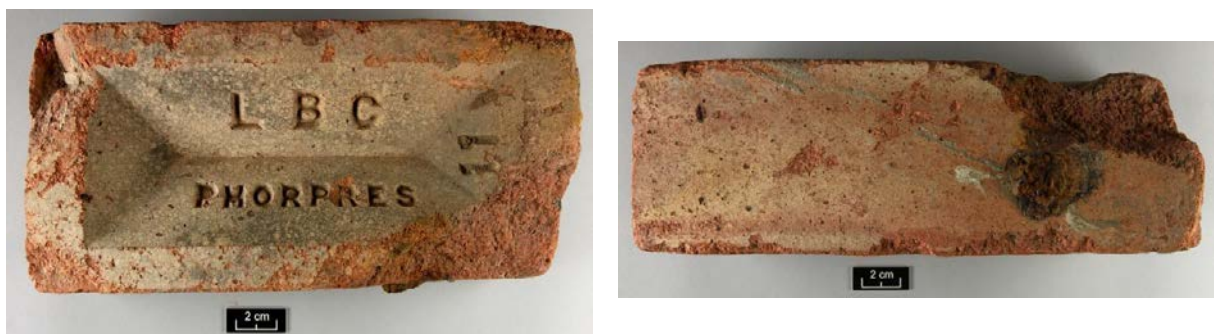
Plate 45: The upper bed and one stretcher of a modern brick from the St Leonard's Hospital excavations bearing the maker's stamp of the London Brick Company
