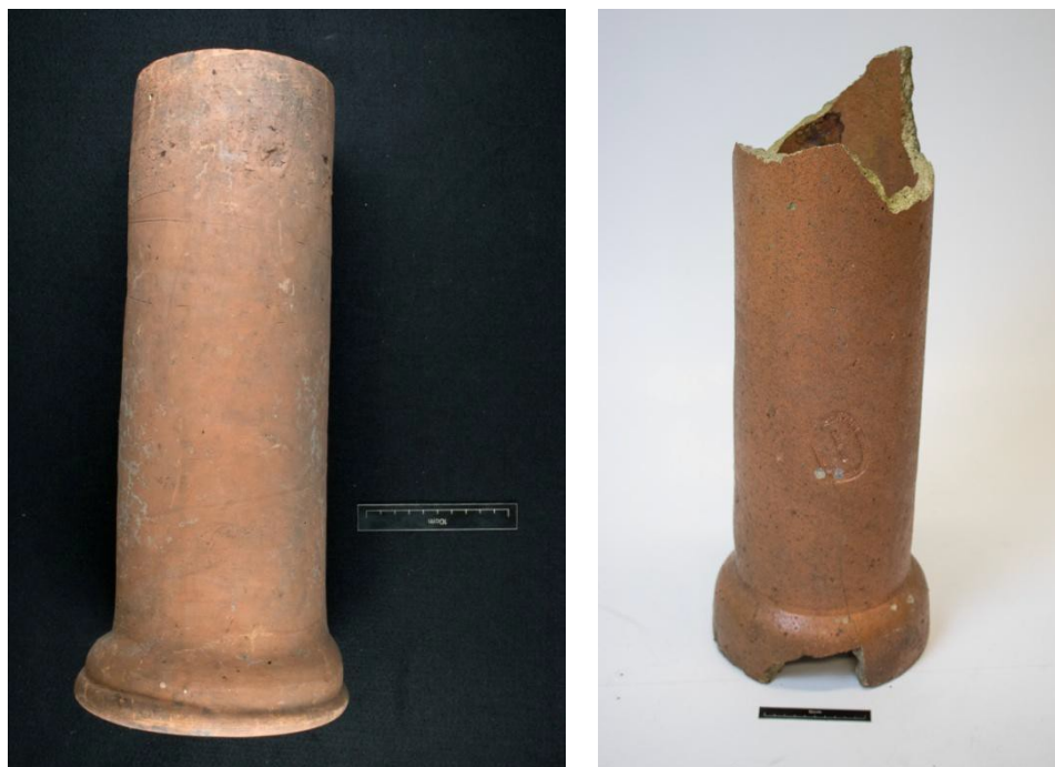
Plate 46: A machine-made drain pipe and salt-glazed sewer pipe from the Hungate excavations, York
