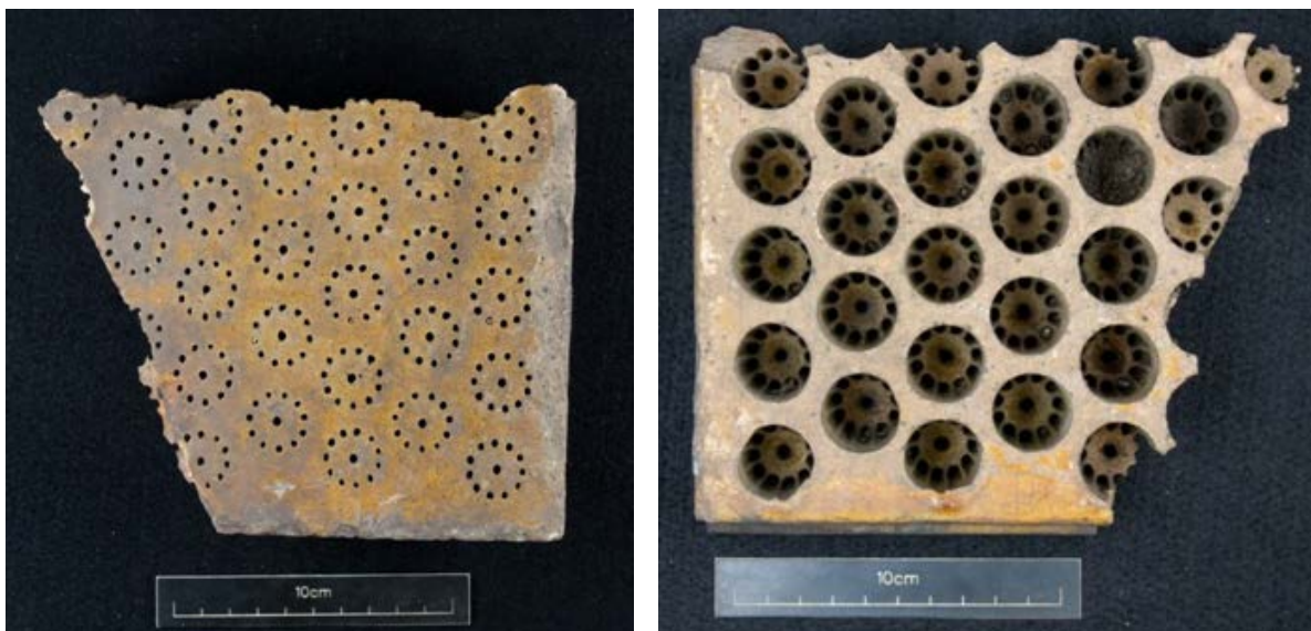
Plate 51: Malting brick from the Clementhorpe Maltings, York
