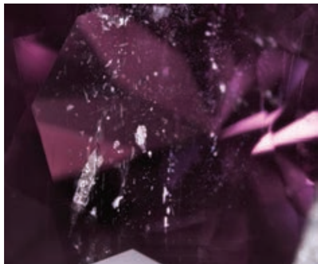
Figure 15: A series of fine, platy negative crystals and thin films are oriented along the basal growth planes in this pink sapphire. Photomicrograph by C. P. Smith; magnified 50 \times .
