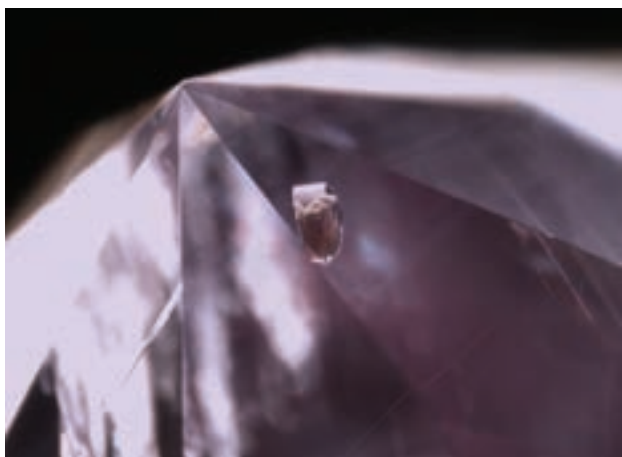
Figure 11: Mica is another of the more common mineral inclusions identified in Greenland rubies and pink sapphires. Photomicrograph by C. P. Smith; magnified 60×.
