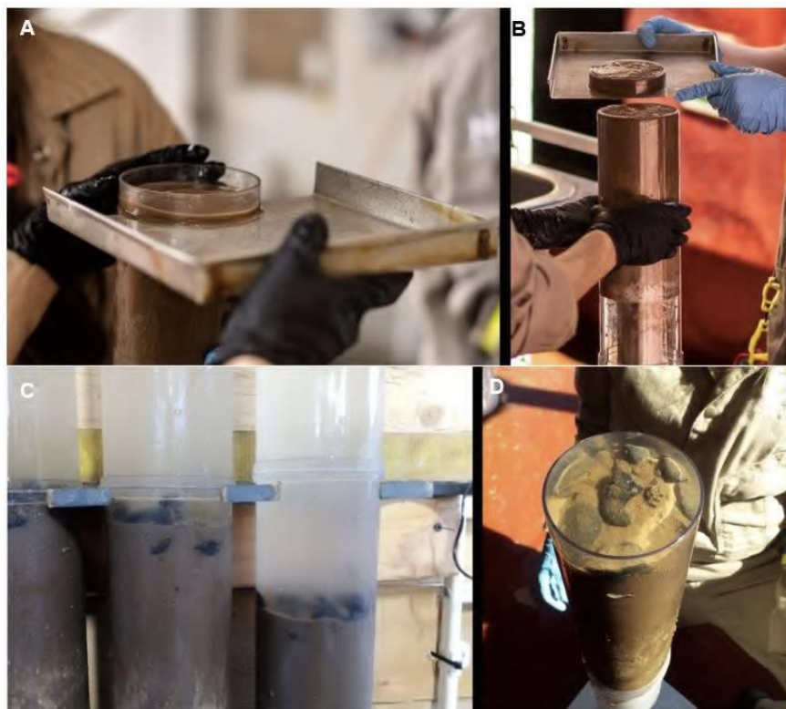
A) Using the aluminium plates, mud was sliced in between the core tube and the slicing ring. B) The plate was slid off the tube with light downward pressure (without pushing the core tube down further onto the extruder), removing the slicing ring and mud with it. C&D) Presence of nodules at the sediment surface and in the deeper sediment layers.
