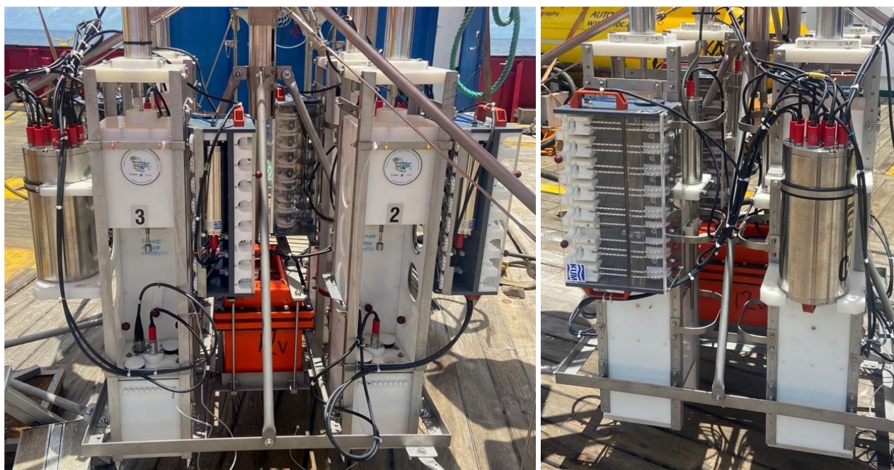
Figure 6-46 Front and side views (right to left) of the benthic respirometer lander used aboard Campaign 5D to conduct in situ incubation experiments
