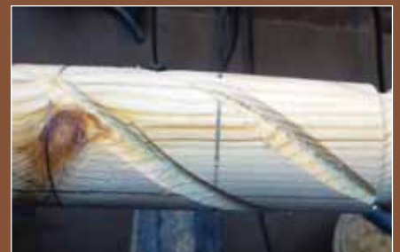
9 - After using the small microplane on the marked out line
