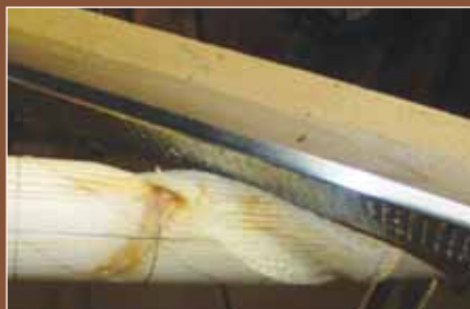
11 - Rounding the edges of the grooves with the flat microplane
