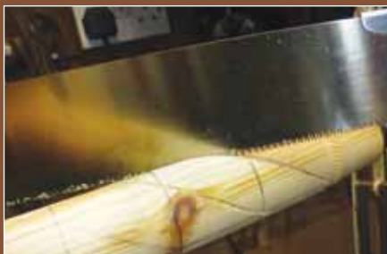
7 - Make the first saw cuts
