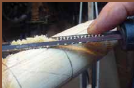
8 - Starting the groove with the small microplane.
