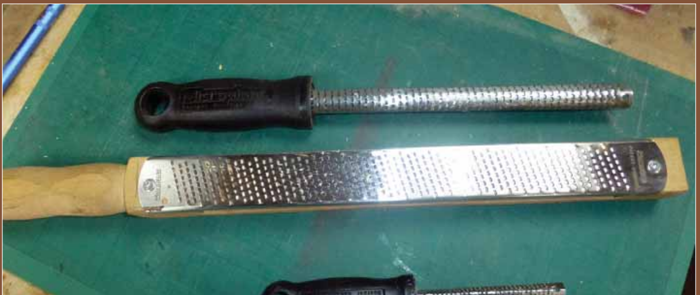
The round, flat and small microplane with the 90 degree edge to start the groove.
