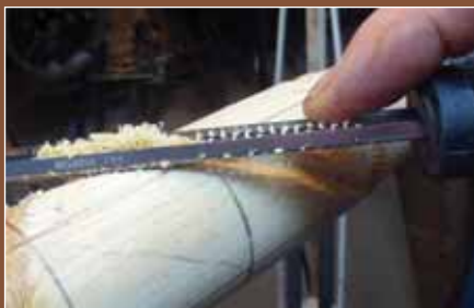
10 - Using a round microplane to widen the groove
