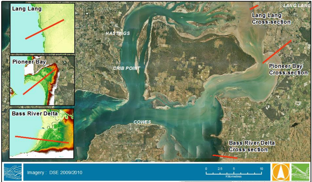
Figure 3-25 Examples of the MHS Tidal Planes Including 0.8m of Sea Level Rise Relative to Low Lying Backshore Plain.
