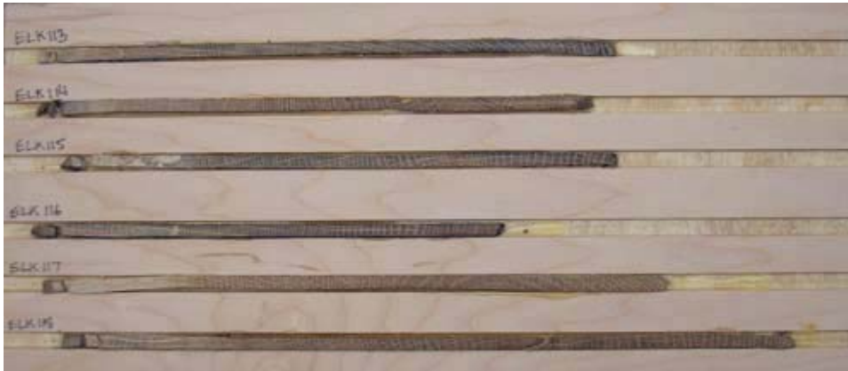
Figure 3.14 Tree ring cores can be used to assess disturbance and changed conditions at a site over the life of the tree. Cores can be taken with an increment borer, mounted, sanded, and viewed with a microscope. Software that measures each annual tree ring is useful for accurately recording small variations in growth and creating site chronologies. Photo: Shyanne Smith
