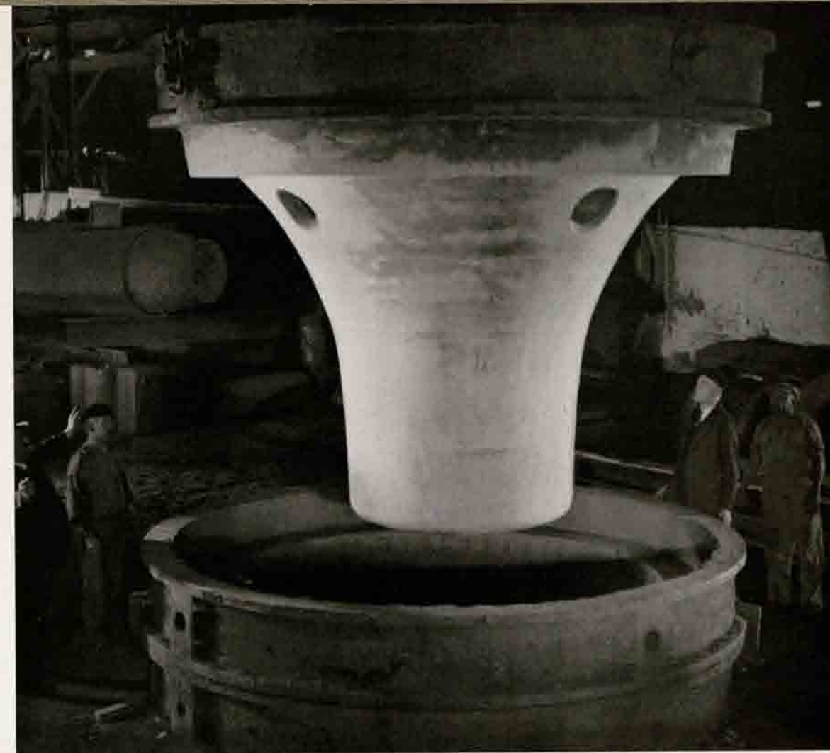
The mould of the core is lowered into the outer form.
