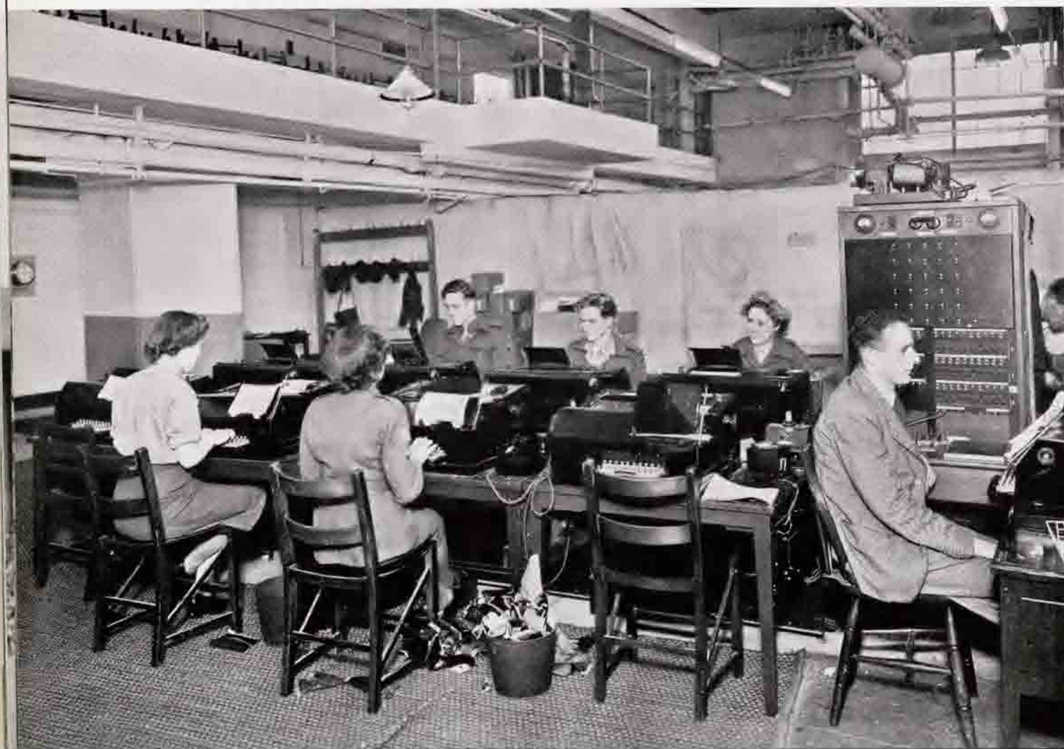
The teleprinter network at Wembley which enabled contact to be kept between the various Olympic offices, arenas and housing centres, and by which results and official instructions and messages were transmitted.
