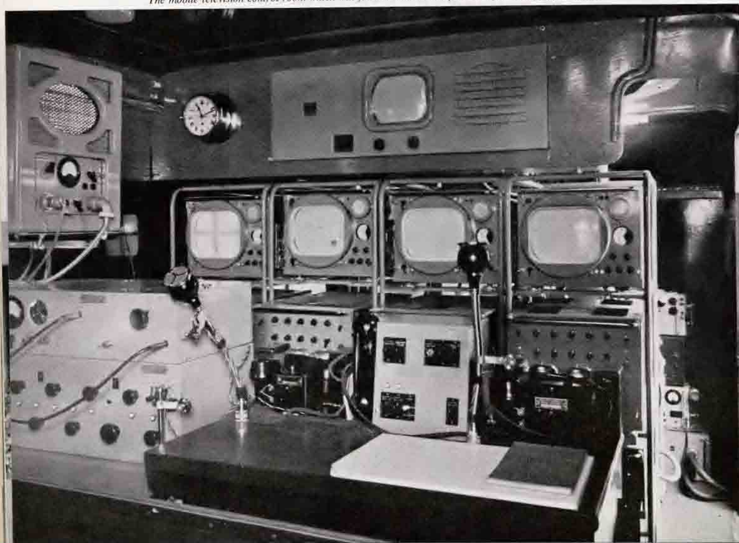
The mobile television control room which was first used at the Empire Pool for the Olympic Games.
