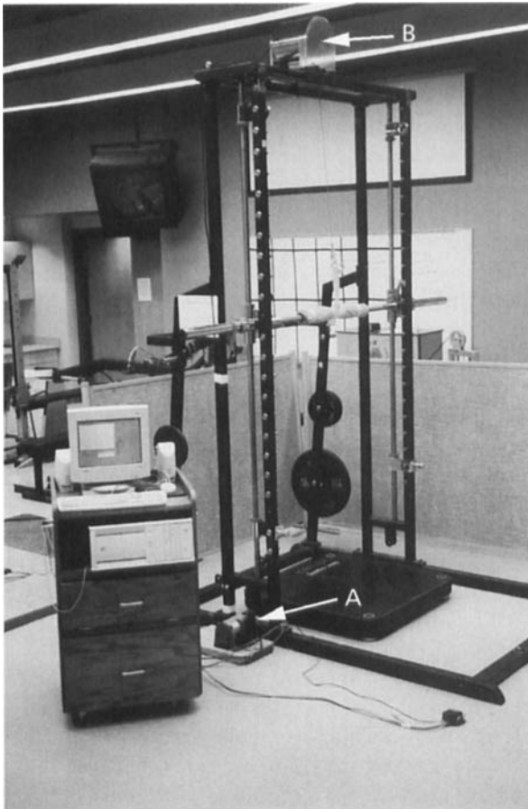
Fig. 3.5 The Ballistic System is an example of the application of the latest technology to strength training. A computer constantly monitors movement of the barbell using a linear transducer (A) providing feedback of force, velocity and power during the athlete's performance. An electronic brake (B) can be used to limit the impact forces and eccentric load on the athlete or to modify the concentric resistance profile.
