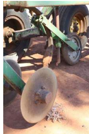
Details of tynes and disc configuration of Mosely’s machine
