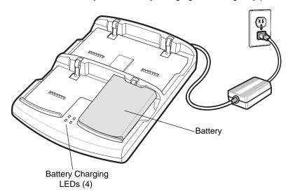
Figure 4-4 Four Slot Battery Charger
