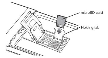
Figure 1-4 Insert microSD Card in Holder
