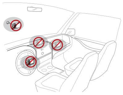
Figure 4-6 Vehicle Holder Mounting
