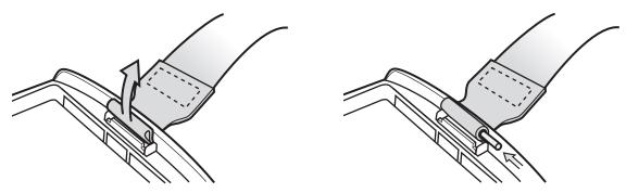
Figure 1-13 Feed handstrap into Handstrap Slot
