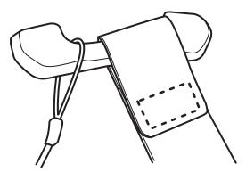
Figure 1-15 Slide Handstrap and Tether Over Handstrap Mount
