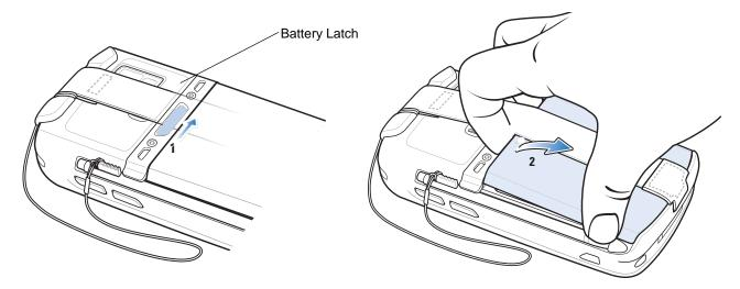
Figure 1-6 Removing the Battery
