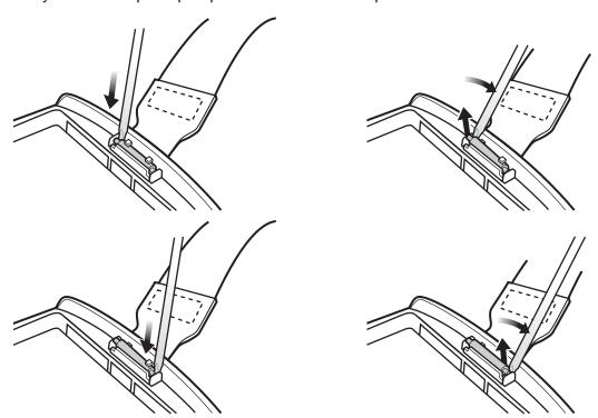
Figure 1-11 Handstrap and Pin Removal
