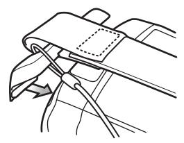
Figure 1-16 Align Mount Bracket with Holes in End Cap
