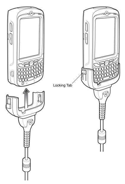
Figure 4-5 Cable Cup Locking Tabs
