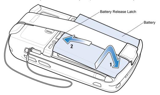
Figure 1-5 Inserting the Battery
