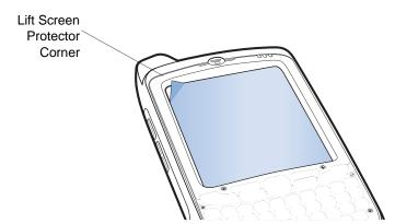
Figure 5-1 Removing the Screen Protector
