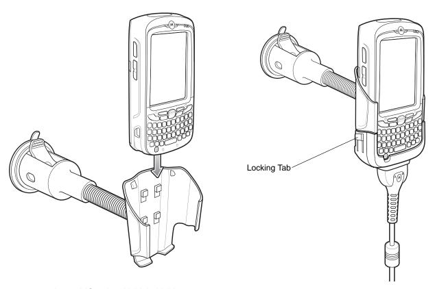
Figure 4-8 Insert MC55 into Vehicle Holder
