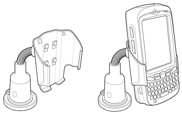
Figure 4-10 Vehicle Holder Mounted on Flat Surface
