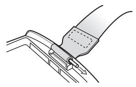
Figure 1-12 Pin Removal
