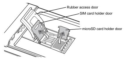
Figure 1-3 Lift SIM Slot Holder Door
