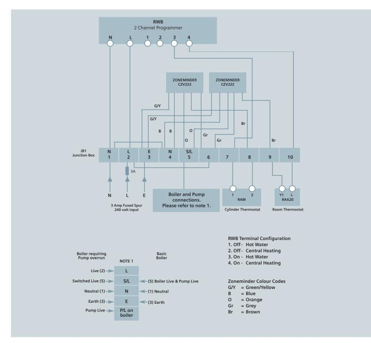
Time and temperature control of Central Heating and Hot Water. Possible to have Central Heating only, Hot Water only or both together.
