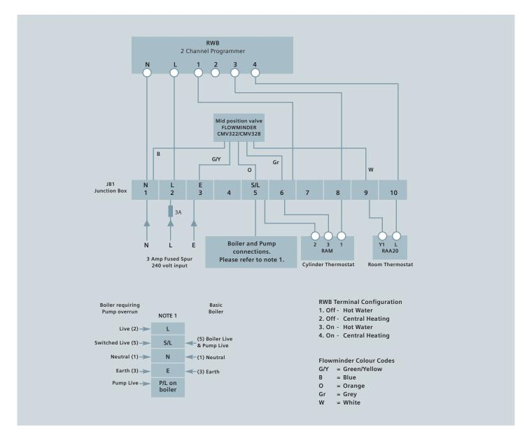
Time and temperature control of Central Heating and Hot Water. Possible to have Central Heating only, Hot Water only or both together.
