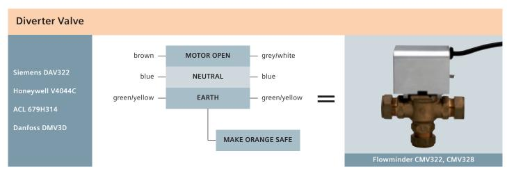
To replace a diverter valve with a mid-position valve, replace old brown wire with grey and white together and make the orange safe.
