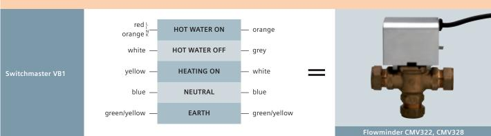
Switchmaster valve is not sprung return hence the extra wire (orange) to move the paddle into the hot water ON position. Insert link on junction box between red and orange of old valve and wire orange to orange.
