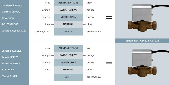
In the event of motor failure all products can be replaced without drain down using DVA actuators (see next page)
