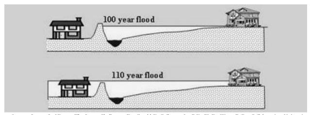
Figure 4-40 Flooding from Levee Overtopping
