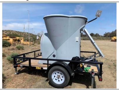
**Figure 2-5**. The SODAR upper-air measurement station is located near the southeast corner of Oceano Dunes SVRA. The co-located 10-meter meteorological tower and the Phillips 66 refinery are shown in the back left of the photo. UCSB and ASU operate the station.
