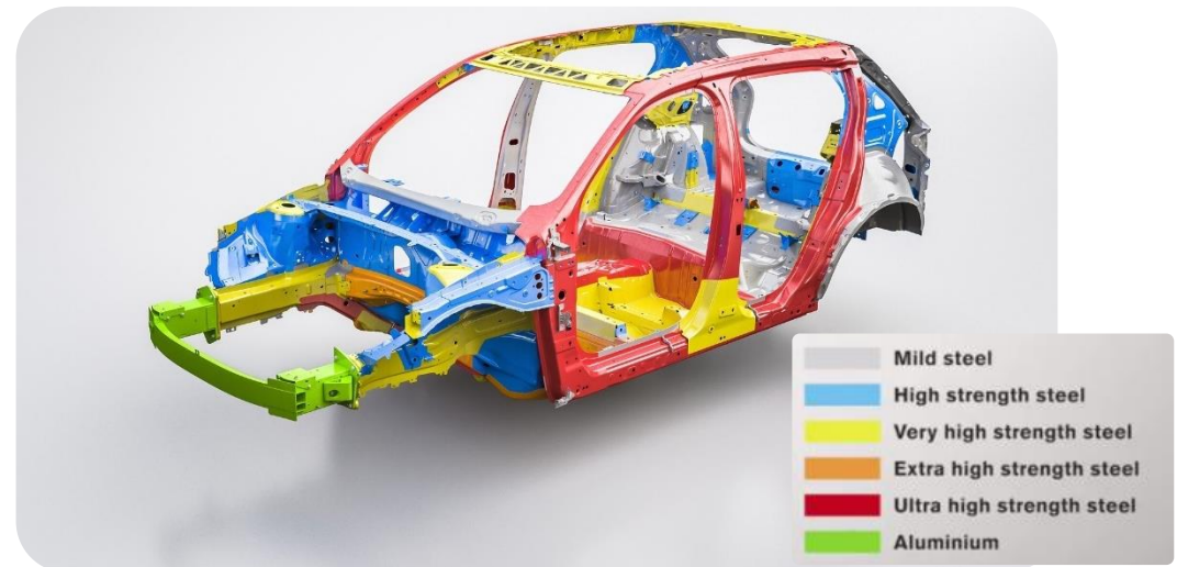
AHSS makes up most of the XC40's safety cage [Images courtesy Volvo Car Group]
