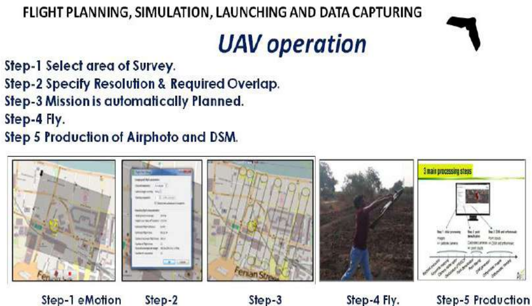
Figure 1.2.1: Mapping Workflow of UAV system
