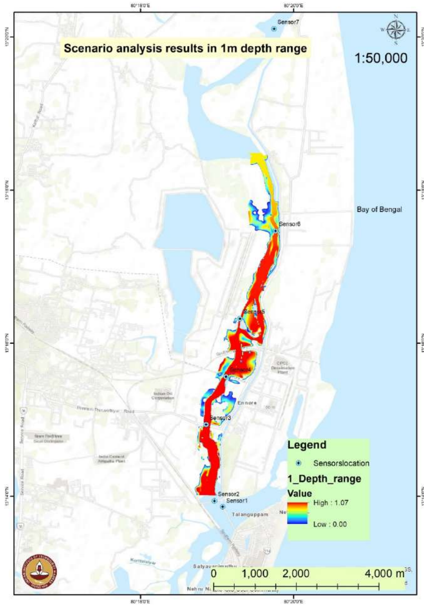
Figure 1.3.24: Tidal Fluctuation range – 1 m dredging
