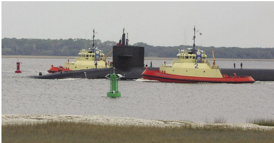
At Kings Bay, Georgia, two buoys containing radiation detectors guard the marine entrance as part of a demonstration project sponsored by the Defense Threat Reduction Agency.
