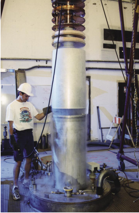
Livermore physicist Darin Kinin helps guide the experiment tower containing the microwave cavity and amplifiers into the magnet bore.
