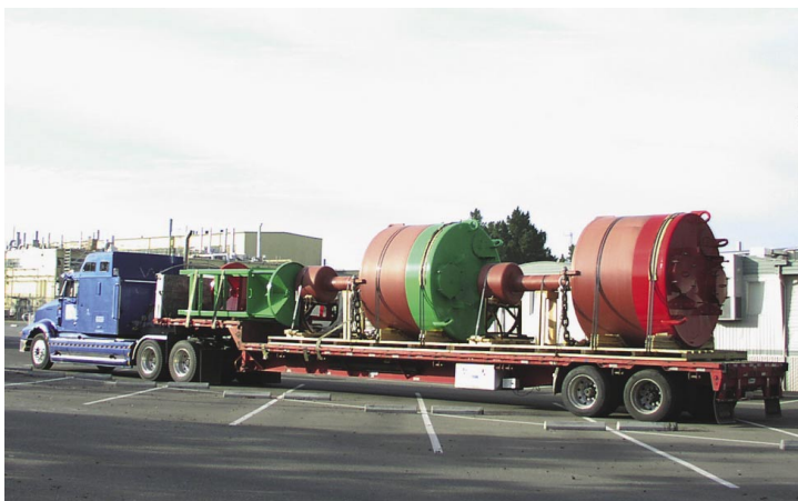
Two commercial stainless-steel buoys, one painted red and the other green, were manufactured in Houston and delivered to Lawrence Livermore on Thanksgiving weekend 2002 for modifications. The buoy towers, which were attached in Kings Bay, are visible just behind the cab.
