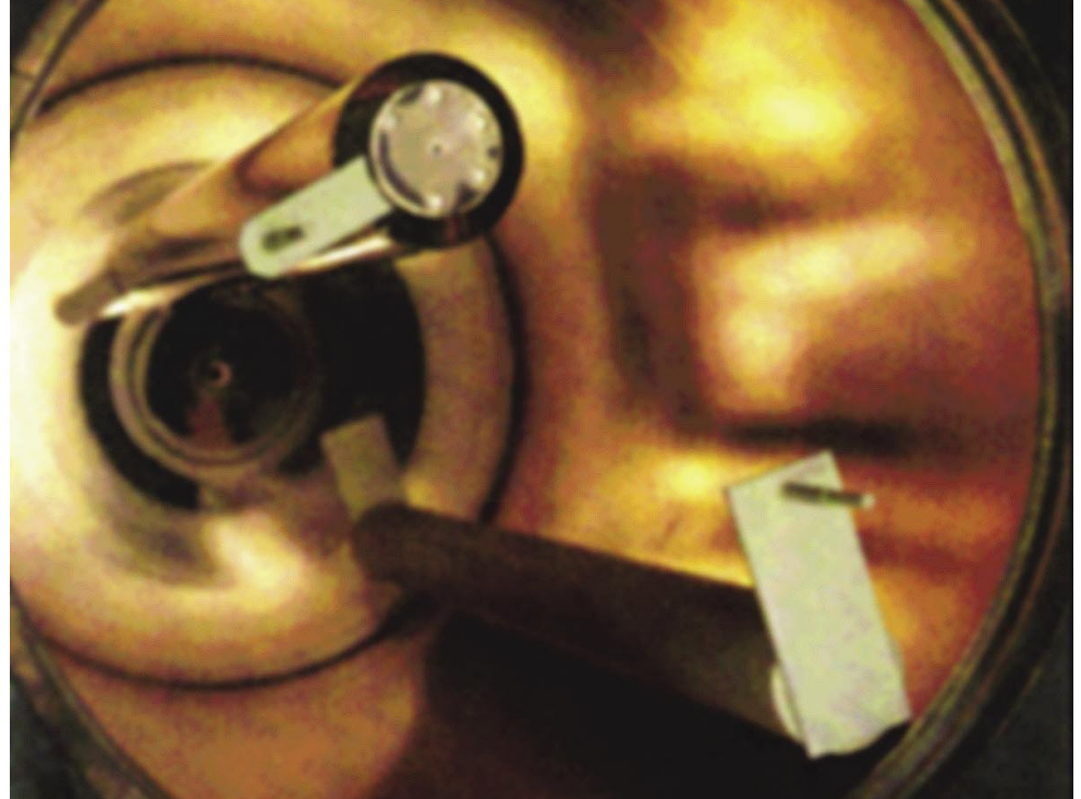
The view from above the axion experiment's resonant cavity shows the inside of a copper-lined cylindrical cavity (50 centimeters in diameter and 1 meter deep) and two tuning rods.
