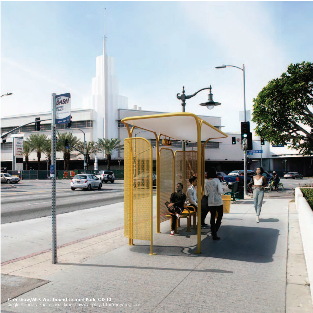
Pairs of columns are tied together with steel connector rings. Up to three additional columns supporting shade panels or lean bars, are bundled together to form one cluster that sits on a base plate.
