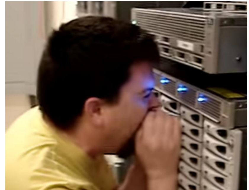
Vibration can badly influence disk latency
