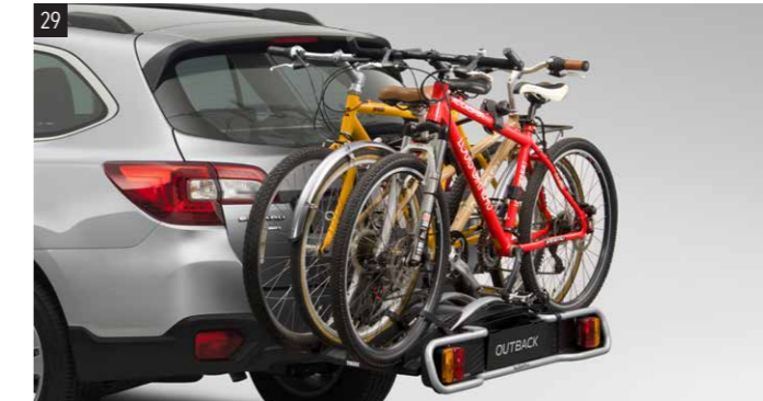
29 Rear Bicycle Holder 3bike 13pin E365EFJ400 Transports 3 bikes on the tow ball. *Trailer hitch required. Max. weight: 1 bike - 20kg, 3 bikes - 45kg.
