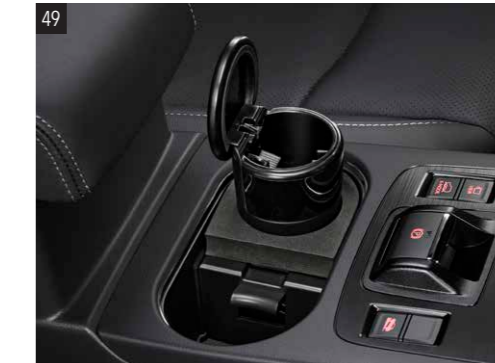
49 Ash Tray (In Cup Holder) 92172AG040 Convenient interchangeable ashtray fits into the center console cup holder.
