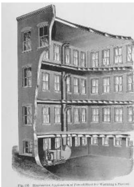
Fig. 136. Illustration of Forced Heat by Watering & Piping.
