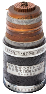
Japan's first single-core 66 kV OF 675 mm 2 cable
