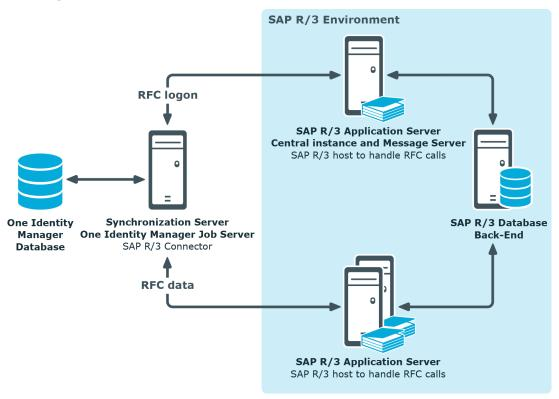
Figure 3: Architecture for synchronization - Communication through router
