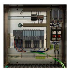
Configuration example SIMATIC ET 200SP HA for distributed configuration: 8 x I/O modules, up to 128 x I/O signals, stainless steel enclosure, dimensions  $600 \times 600 \times 300$  mm (width x height x depth)
