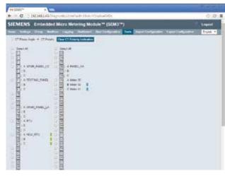
Diagnostics: Displays all active metering and can provide metering Modbus Register information
