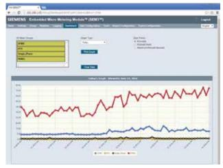
SEM3 now includes a dashboard within the controller. Trending of multiple points at the same time allows the user to compare energy consumers and refine their systems or identify anomalies targets for correction.
