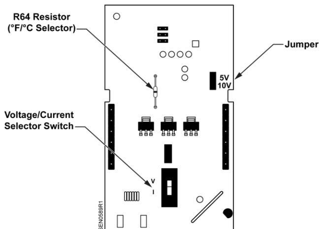
**Figure 4. Circuit Board**
