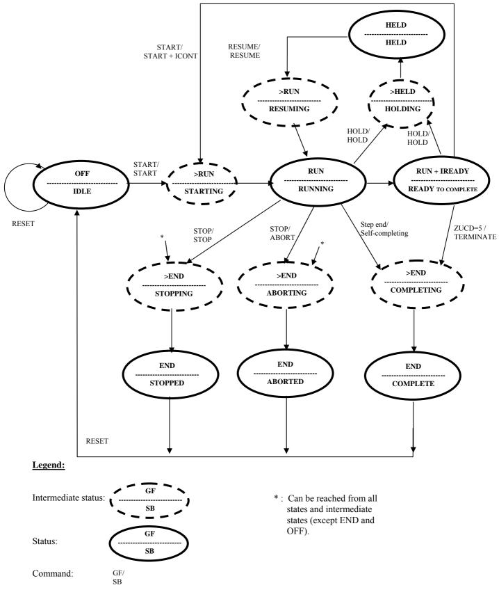
The intermediate statuses relate to the GF (GF block) but are not indicated in the SB (interface block).
