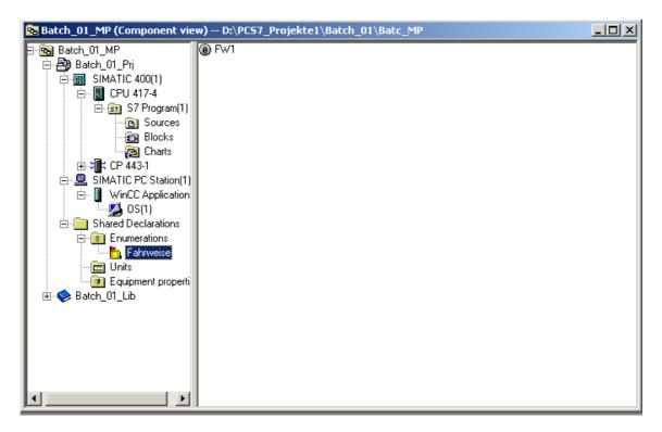
Via "Properties" FW1 enter value 1. Configure the same way for FW2 ... FW6 (value =  $2 \dots 6$ ).
