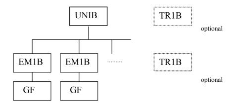
The schematic shows the basic structure of the blocks required on the AS for use with SIMATIC BATCH.
