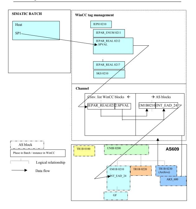
This figure shows how the channel works based on the example of a write job for the first setpoint of the "Heat" function. At the same time, the naming convention is illustrated in a practical situation.
