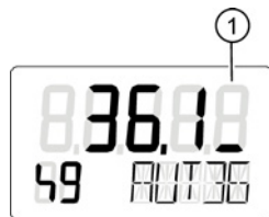
Figure 9-4 Display of a threshold 1 fault message
