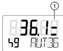
Figure 9-5 Display of a threshold 2 fault message
