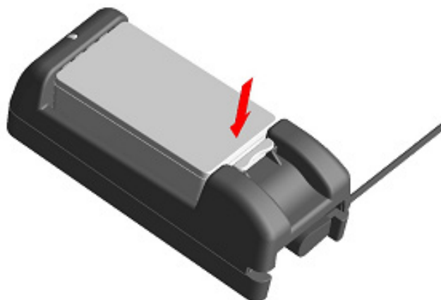
Figure 17-6 Battery Pack Installation (2)
