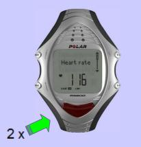
The stopwatch starts, a heart symbol blinks and the horse's heart rate is displayed in the bottom of the screen. From now on, the RS800CX is recording your exercise.
