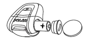
Use a coin to unscrew and open the metal battery cover. Place the LR6 battery as indicated and screw the metal cover back into place.
