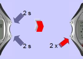
Press and hold UP for 2 seconds to zoom in the data of the top row, or **DOWN** for 2 seconds to zoom in the data of the bottom row. Press and hold the same button for 2 seconds to zoom out.
