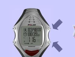
To check the data you are most interested in, change display by pressing UP or DOWN. (6 different displays are set by default but can be customized - see user manual)
