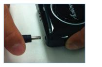
**Note**: Use the 5V/2A power adapter provided by Actiontec (Model # WA-10P05FU) only.
