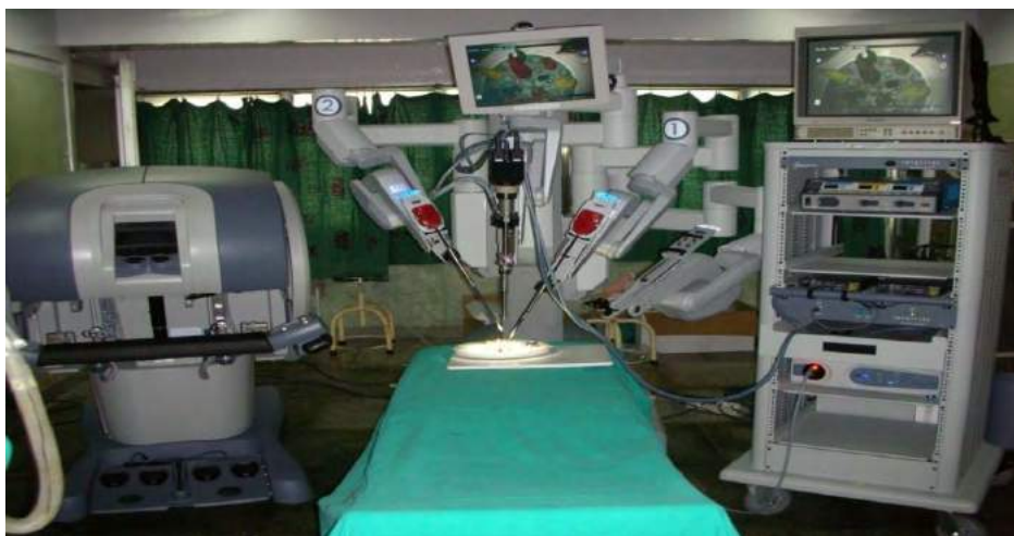
Figure 7: da Vinci Xi robotic system
