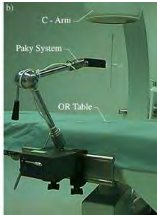
Figure 3: the AcuBot used to place needles for thermal ablation into renal parenchyma percutaneously
